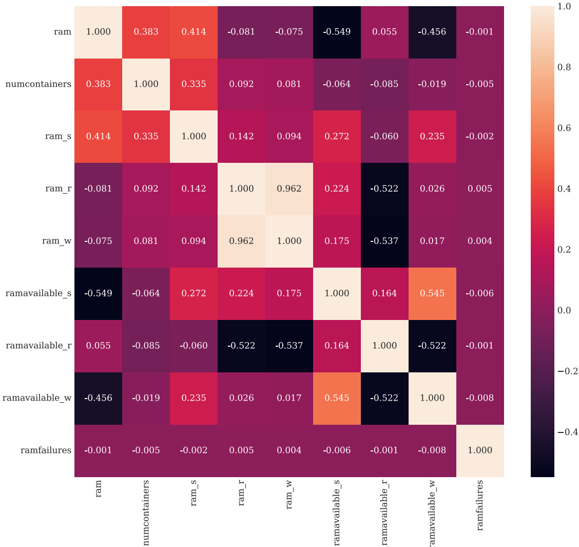
Figure A.2: Correlation matrix of the RAM metrics collected from the hosts in scenario 1.
